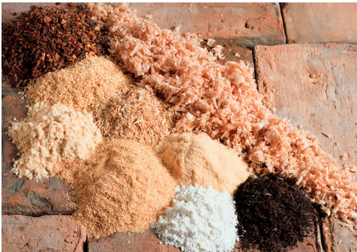
Figure 42: Example of feedstock for WPC production
