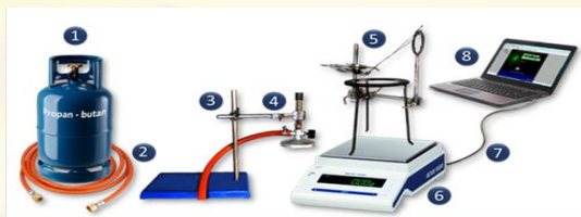
Description: 1- gas cylinder, 2- gas intake tube, 3- burner holder, 4- burner, 5- sample holder, 6- scales, 7- connection between scales and computer, 8- computer
