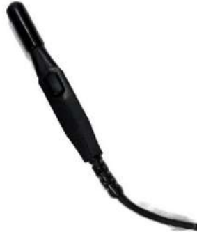
Figure 7. Stylus is a pen used to record the coordinates of an object in a given space.
