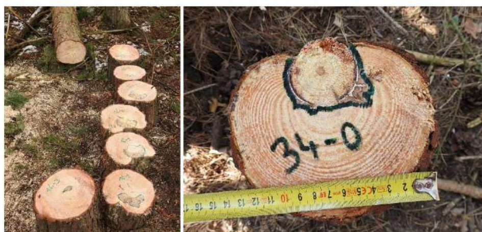
Fig. 2. Scots pine trunk crosscuts and highlighting the rot-damaged area.
