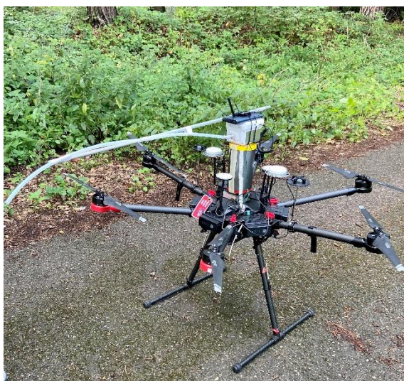
Figure 2. Electronic nose Sniffer as a payload on the DJI Matrice 600 Pro drone with 1 m long Teflon tube for data collection (Hüttnerová et al., 2023).
