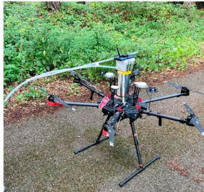
Figure 4. Electronic nose Sniffer 4D placed on multi-copter DJI Matrice 600; Teflon meter tube was used for sampling air.
