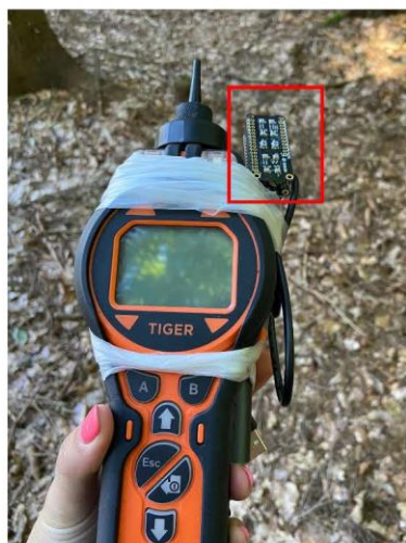
FIGURE 3 On the left side is Handheld VOC Detector Tiger, in the upper right in the red rectangle is Miniature Bosch sensor device.
