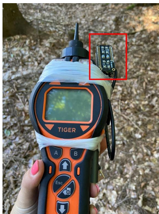
Figure 3. On the left side is Handheld VOCs Detector Tiger (is described below in section 4) Handheld VOC Detector Tiger), in the upper right in the red rectangle is Miniature Bosch sensor device (Hüttnerová and Surový, 2024).
