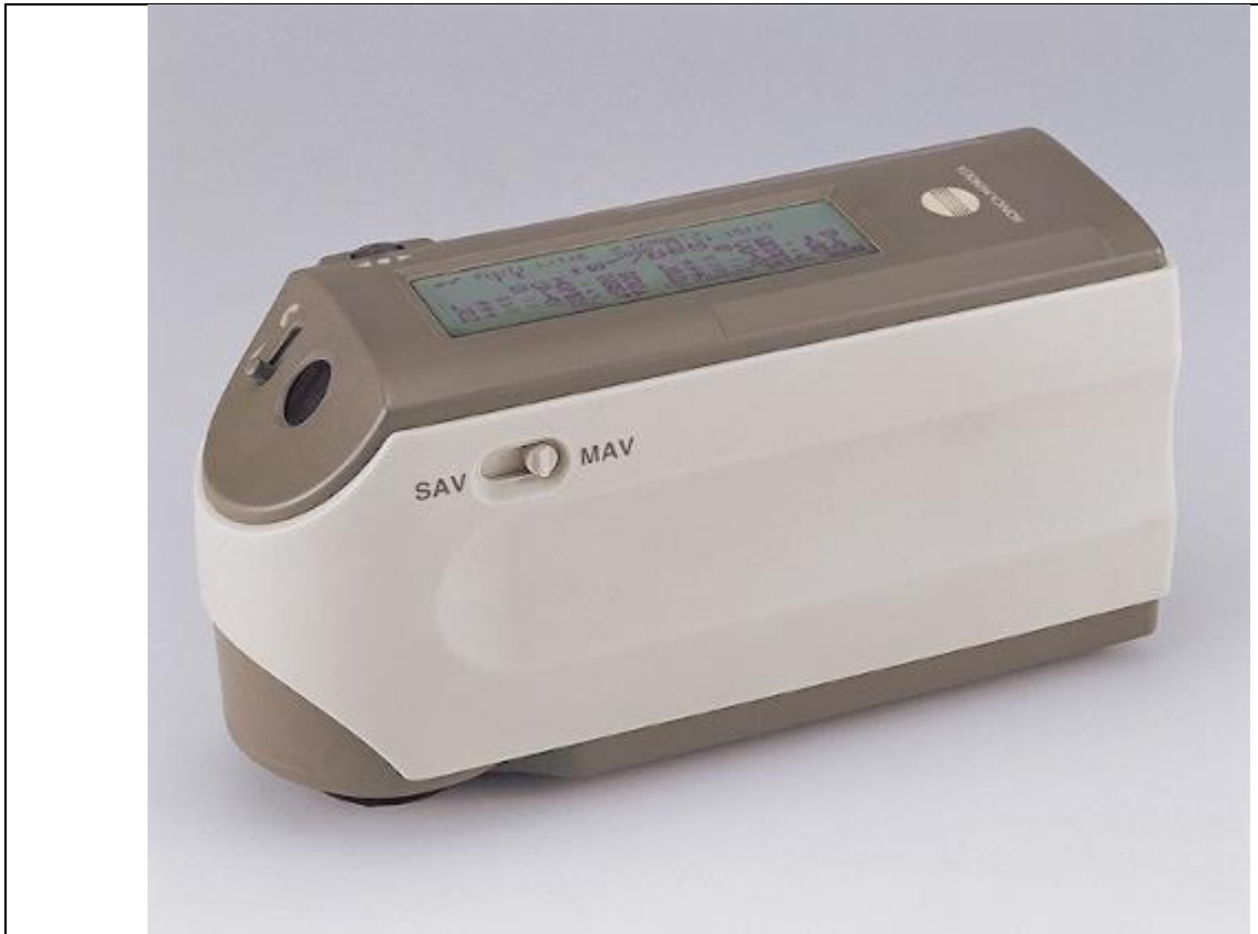
Figure 19. Color measurement using a spectrophotometer (©2006–2025 Konica Minolta Sensing Americas Inc.).
