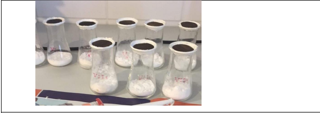
Figure 29. Laser cut beech samples prepared for diffusion test according to ISO 12572:2016.
