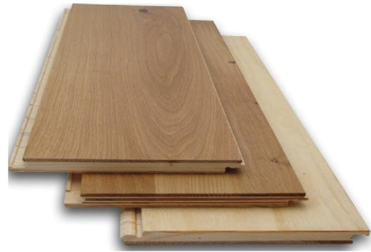
**Fig. 1.** Examples of some of the wood products used in this study. Samples (from left to right, up to down): 3-layer solid wood flooring (upper layer: 0.3 mm UV-curable layer, 3.8 mm oak veneer; core: 8 mm spruce wood; bottom layer: 2 mm spruce veneer); engineered flooring: 0.3 mm UV-curable layer, 3.8 mm fancy oak veneer and 8 mm plywood; 3-layer solid wood flooring: bottom side.
