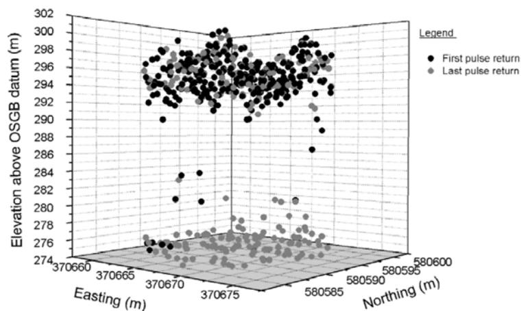
Figure 2. Distribution of first and last LiDAR pulses (from DONOGHUE et al. 2006)
