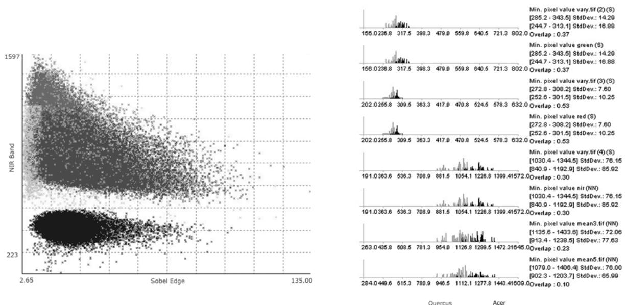
Figure 14a, 14b. Two-dimensional scatter diagram plotting Sobel Edge (horizontal axis) versus NIR band (vertical axis) Histogram representation of two different classes for various classification features.
