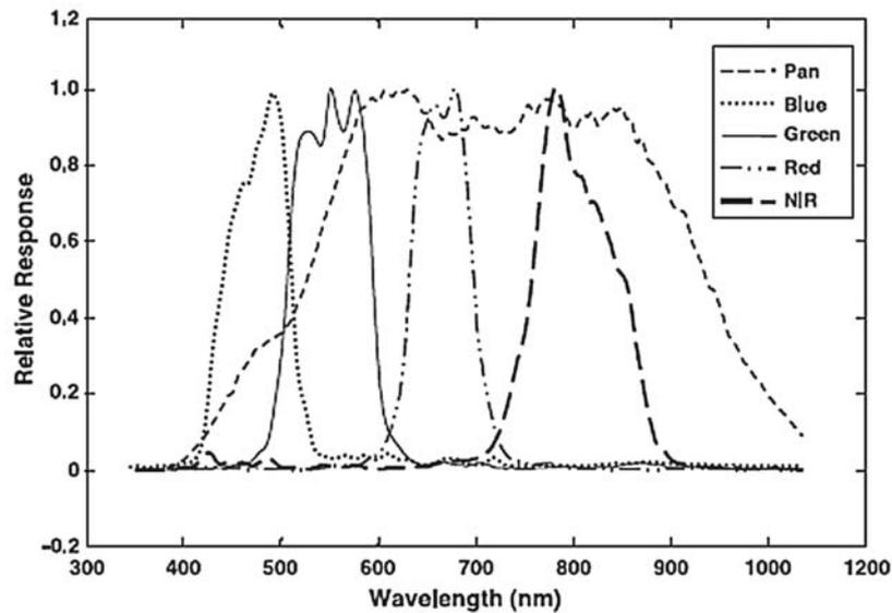
Figure 9. The relative radiometric response of the IKONOS multispectral imagery
