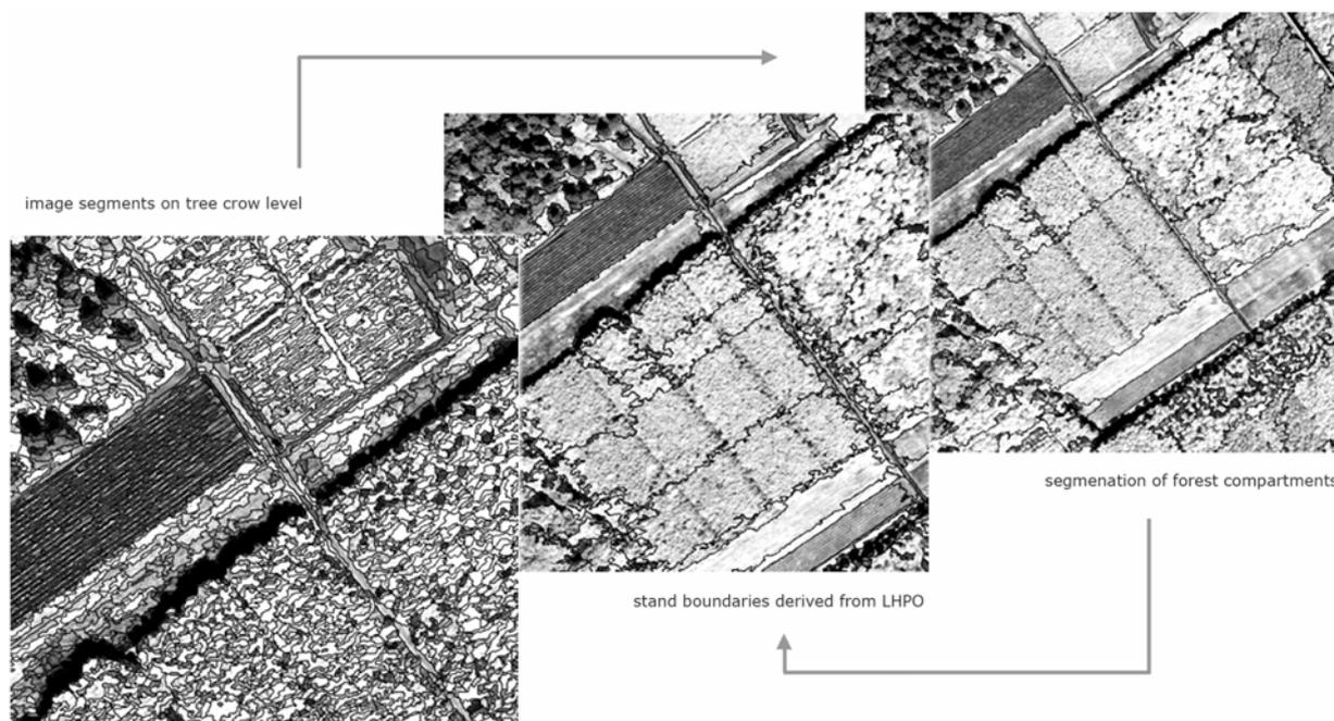
Figure 5. Bottom-up segmentation at three image object levels - tree crowns, GIS-based stands and forest compartments.
