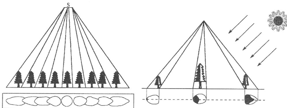
Figure 3: Canopy shape in connection to position in the image and the sunlight direction (ŽÍHLAVNÍK and SCHEER, 2000)
