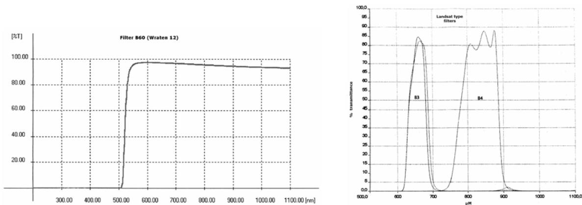
Figure 2. Transmittance custom-made optical filters B60 (Wratten 12) and Landsat type B3 and B4 (Optical research workshop AV Turnov 2002)
