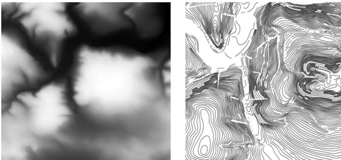
Figure 1. High resolution digital elevation model (left) calculated from ZABAGED® (COSMC) digital contours (right)
