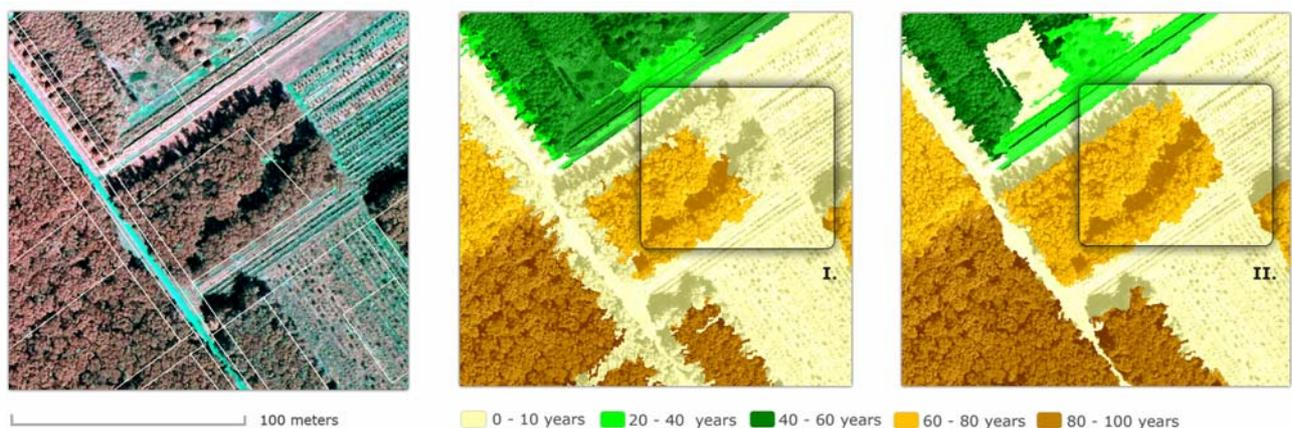
Figure 8. The process of subsequent update of existing GIS layer. Image segmentation and classification based on thematic input (I.) and the class boundary improvement resulting from the multilevel class relations
