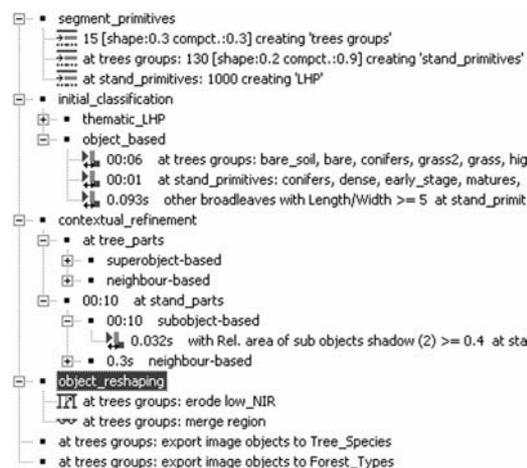
Figure 6. The image analysis workflow in form of process tree: The initial multi-level segmentation followed by “crisp” and fuzzy classification algorithms and class-related refinement. The last phase represents improvement of the object border and conversion into GIS thematic layer.
