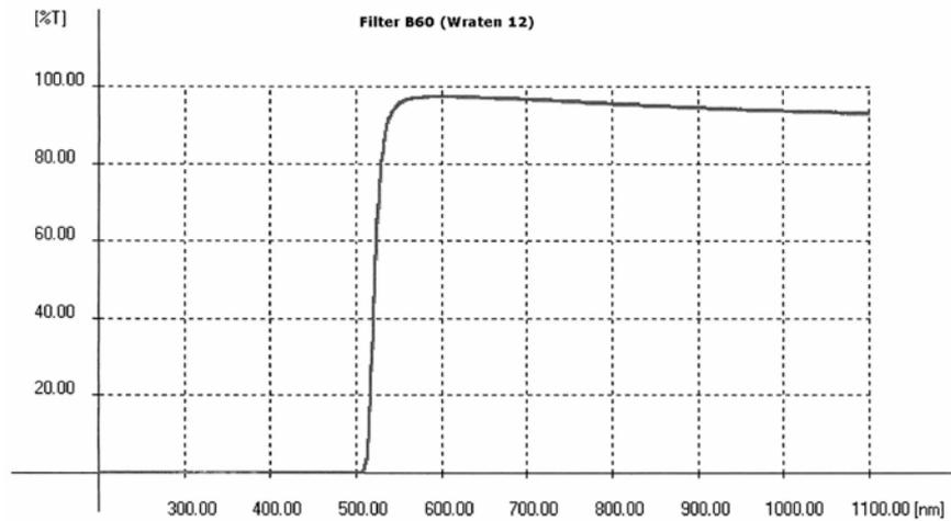
Figures 11a, 11b. Transmittance custom-made optical filters: Landsat type B3 and B4 and B60 (Wratten 12) (Optical research workshop AV Turnov 2002)
