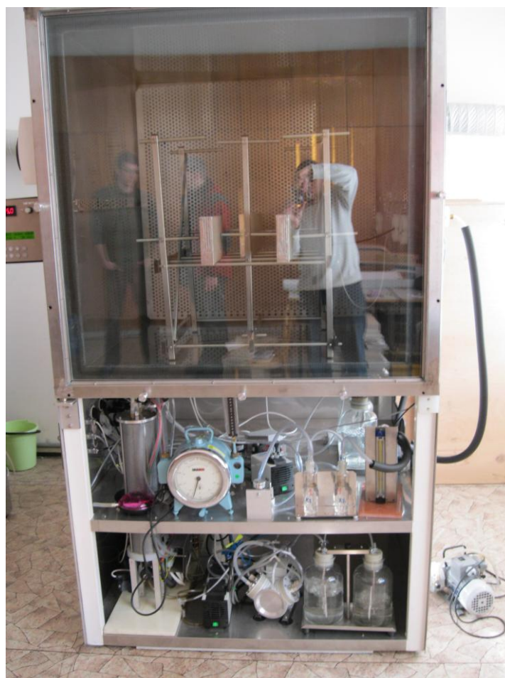
Figure 8: American small-scale chamber (1 m 3 ) used for determining formaldehyde concentration in air from wood products.
